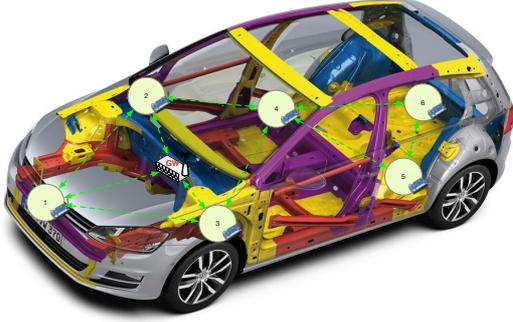
Fig. 1. Multi-hop Intra-car Wireless Sensor Network
