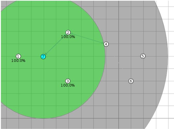
Fig. 3. COOJA Simulation Environment with Unit Disk – Distance Loss Radio Model and RPL-UDP Communication
