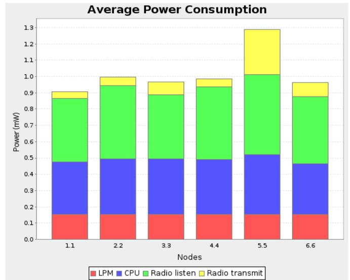
Fig. 4. 6 Node IPv6 WSN Simulated Average Power Consumption
