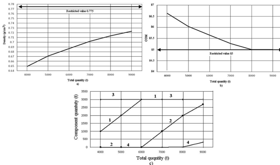
Figure 3 a) commercial gasoline density; b) Motor octane number c) commercial gasoline composition: 1 – FCC gasoline; 2 – catalytic reforming gasoline; 3 – iC5 fraction; 4 – bioethanol.
