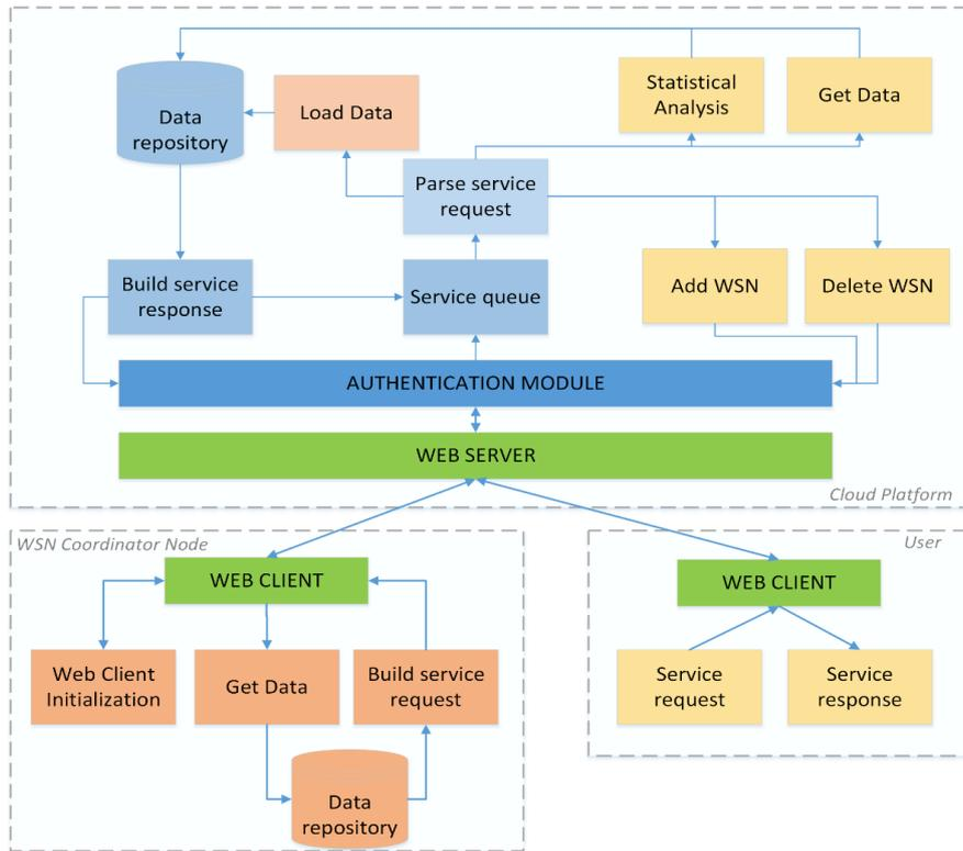
Fig. 1. Inter-module communication for IWSN integration in a Cloud Platform
