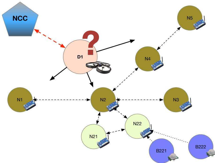
Fig. 1. System diagram for UAV-supported cluster head data collection
