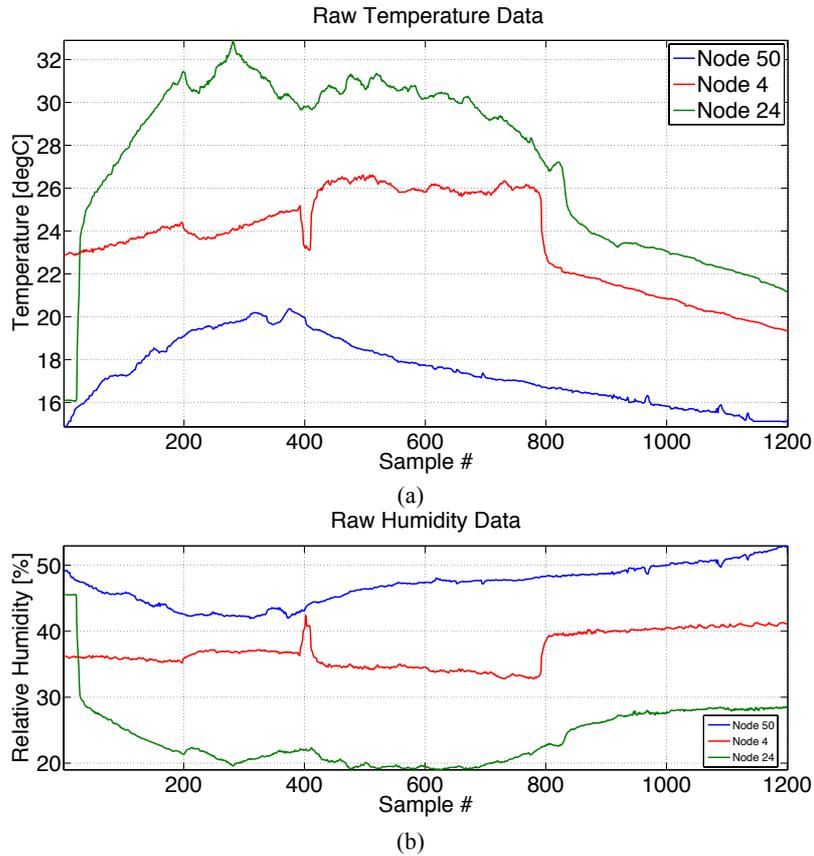
Fig. 2. Raw data collected from the sensor nodes (a) temperature and (b) humidity
