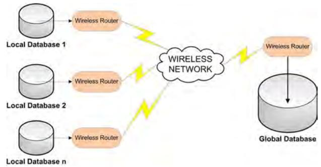
Fig. 2. Wireless communication between the local and the global database
