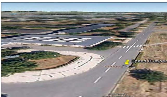
Fig. 4. Speed bumper (one of the possible infrastructure entities that can be mistaken for a road defect)
