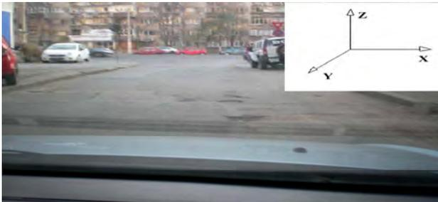
Fig. 6. Accelerometer axis orientation and potholes as seen from the interior camera deployed on a vehicle
