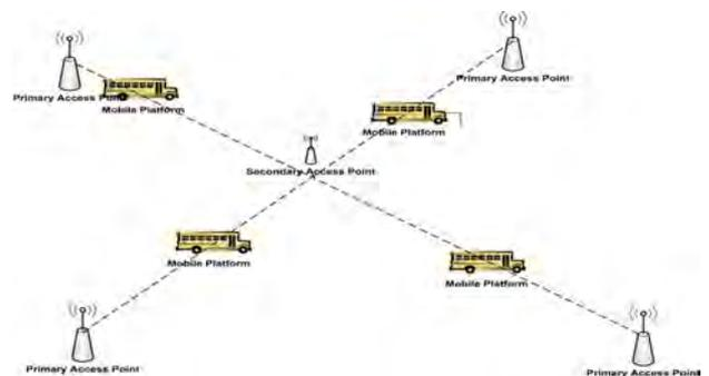
Fig. 3. Primary and secondary access points placement in an urban scenario
