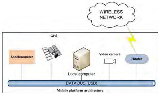
Fig. 1. Mobile platform system architecture
