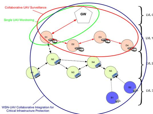
Fig. 1: General collaborative large scale monitoring system based on WSN-UAV integration
