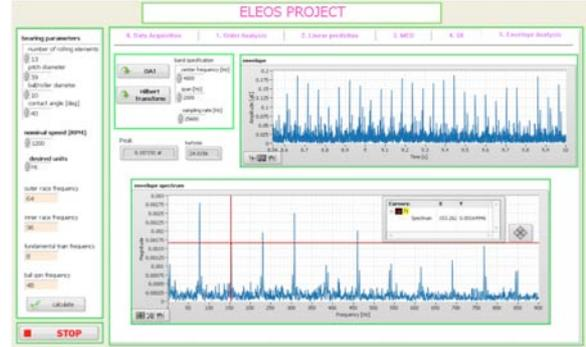
Fig. 5. ELEOS Virtual Instrumentation Project for Envelope Analysis
