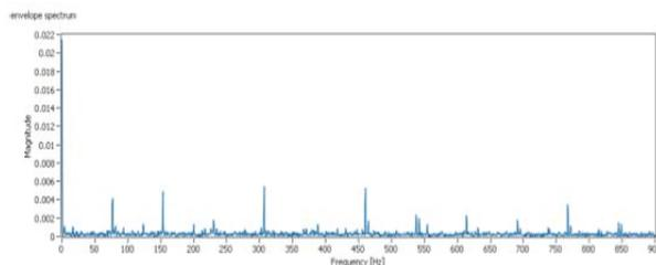
Fig. 8. Envelope Spectrum for the Used Bearing
