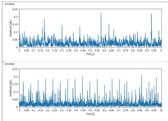
Fig. 7. Working vs. Used Bearing Envelope
