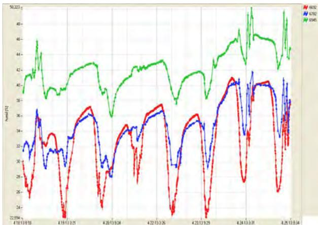
Fig. 9. Humidity Parameter monitored by 3 Nodes.
