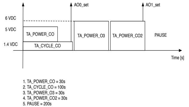
Figure 4. Periodic Sampling of the Gas Sensors
