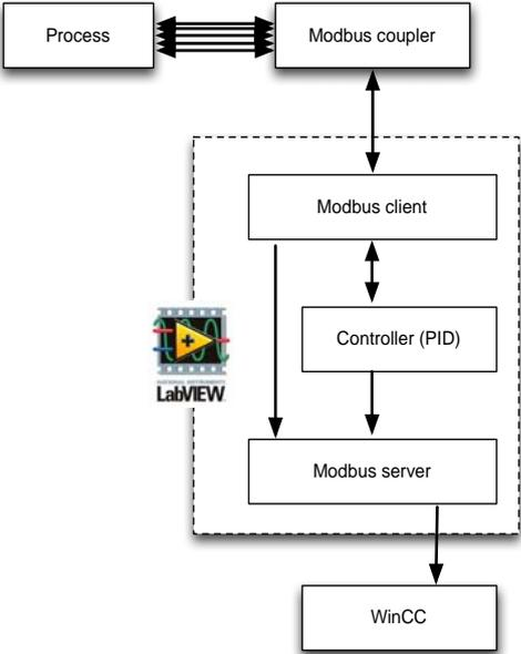
Figure 5. LabVIEW project structure
