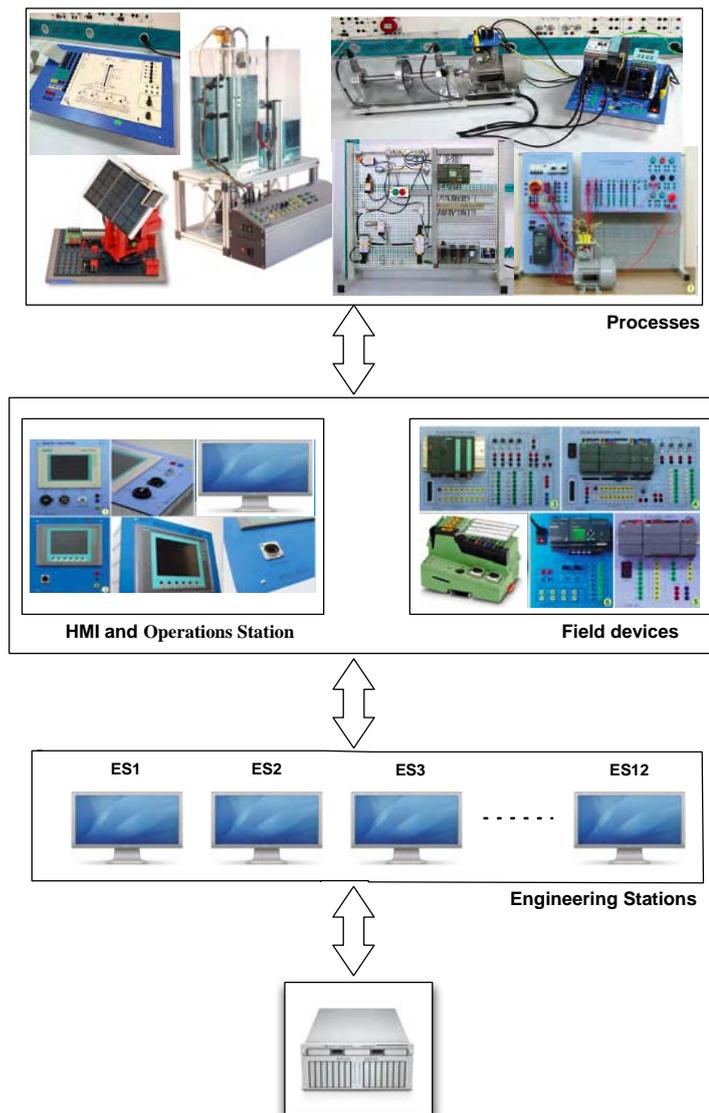
Figure 2. Hardware overview of the laboratory
