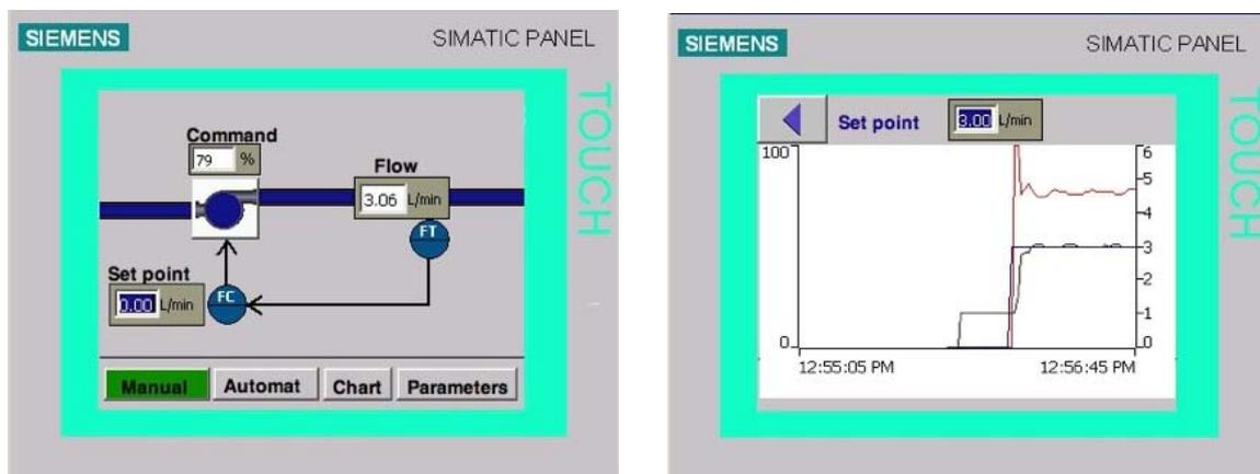
Figure 4. HMI application screens
